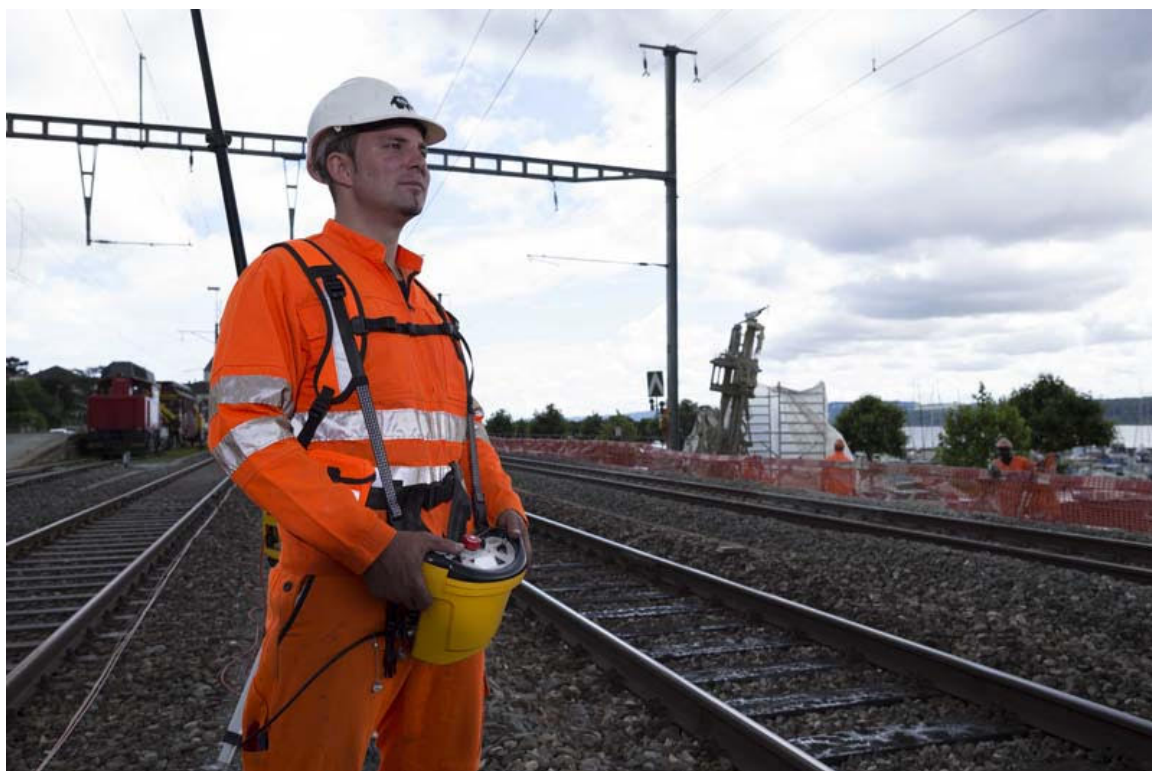
Figure 2 Lookout operated warning device transmitter (photo courtesy of Schweizer)
