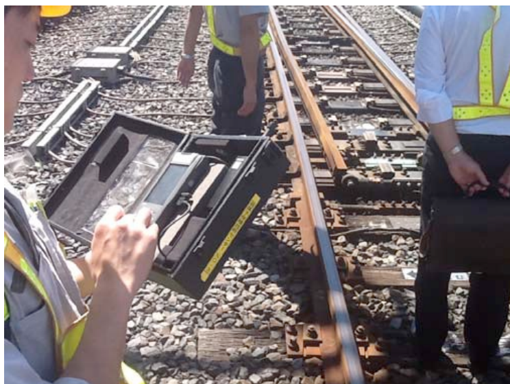
Figure 10 ATOS hand-held terminal (photo courtesy of Nick Thorley, Network Rail)
